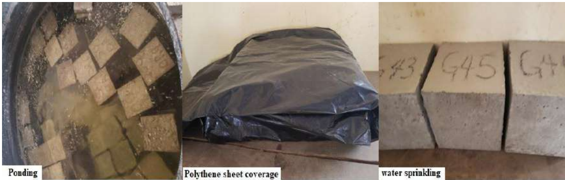
Plate 2: Curing of concrete cubes using ponding, polythene sheet coverage and sprinkling methods
