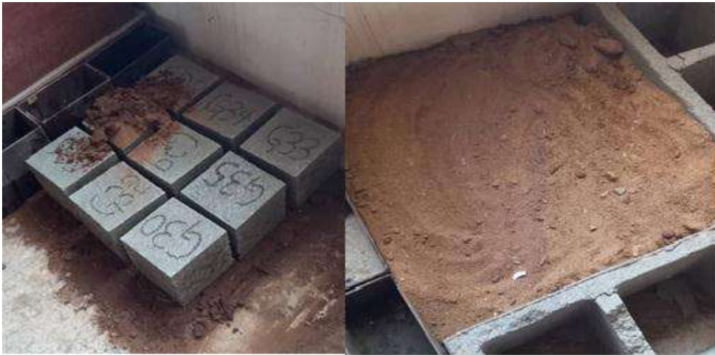
Plate 3: Curing of concrete cubes using sand curing method
