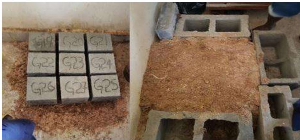
Plate 4: Curing of concrete cubes using sawdust curing method
