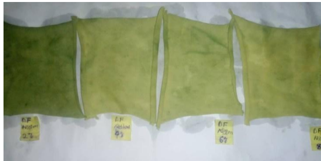
Figure 9: Nylon fabrics dyed with the isolated dye and tested for colour fastness
