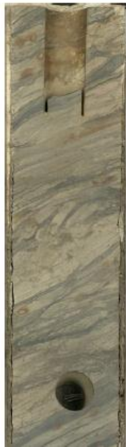
Plate 9: Bioturbated Fine to Medium grained Sandstone (BfmS) Facies (3793-3793.5)
