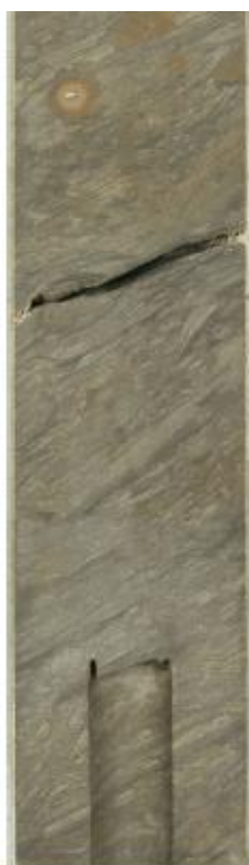
Plate 2: Bioturbated Fine Grained Sandstone (BfS) Facies (3766-3766.5)
