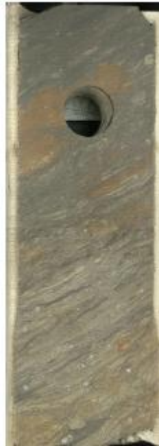
Plate 3: Bioturbated Fine to Medium Sandstone (BfmS) Facies (3769-3769.4)
