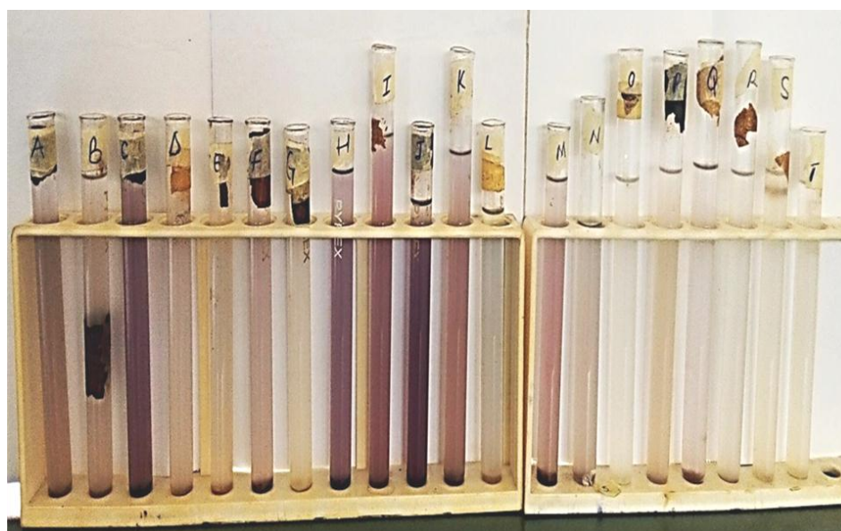
Plate 1: Test tubes showing colour change in relation to potassium bromate composition for the twenty bread samples.
