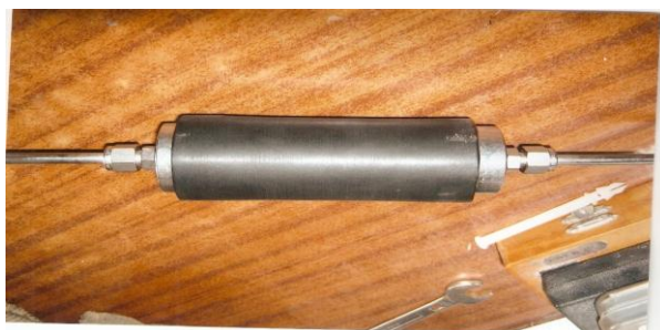
Plate 3: Sample in a Rubber boot with endstems Plate 4: Resistivity core holder and Digibridge
