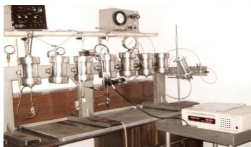
Plate 3: Sample in a Rubber boot with endstems Plate 4: Resistivity core holder and Digibridge
