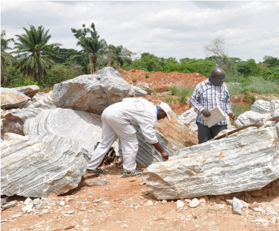
Plate 3: Field photograph of calc gneiss boulders after primary blasting at Igue-Oke (site No. 3)
