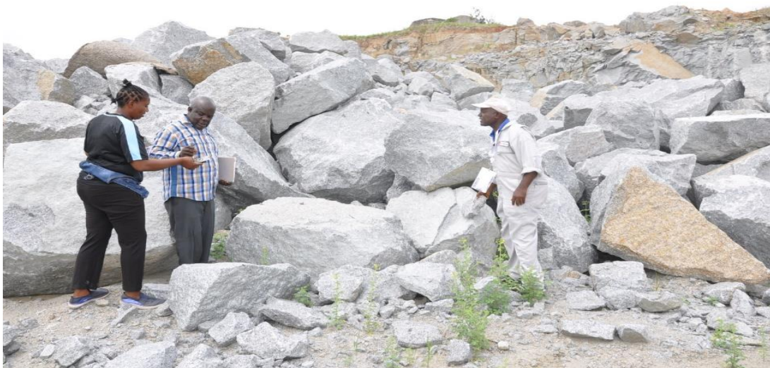
Plate 2: Field photograph showing boulders at Igue-Oke after primary blasting (Site No. 2)
