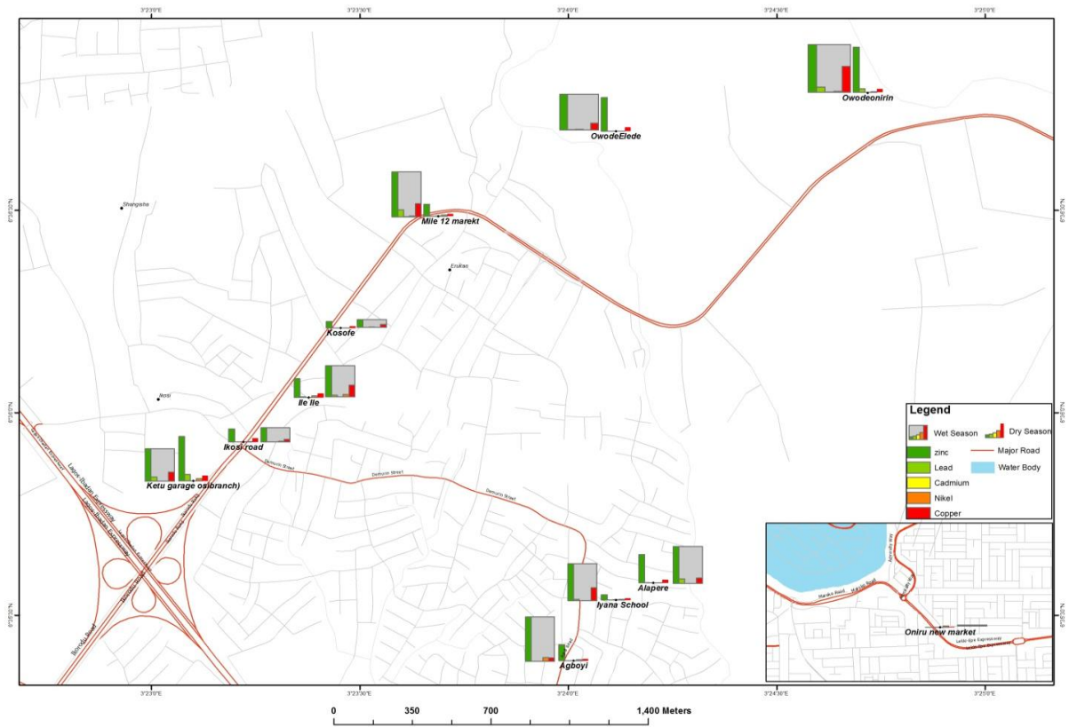
Figure 3: GIS map of Ketu-Mile 12 showing the average mean concentration of heavy metals of each sample sites during the wet and dry seasons.
