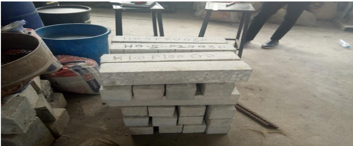
Figure 3: Beam samples before flexural test
