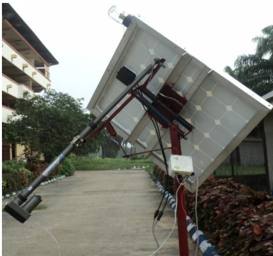
Figure 3: The employed locally constructed dual-axis solar tracker in-situ.
