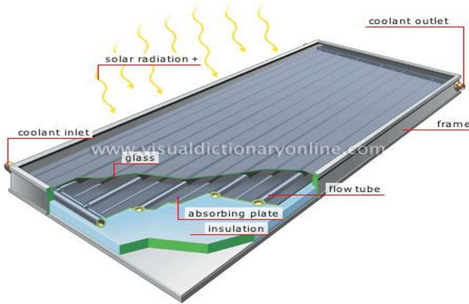
Fig. 1 : A typical structure of a solar panel.
