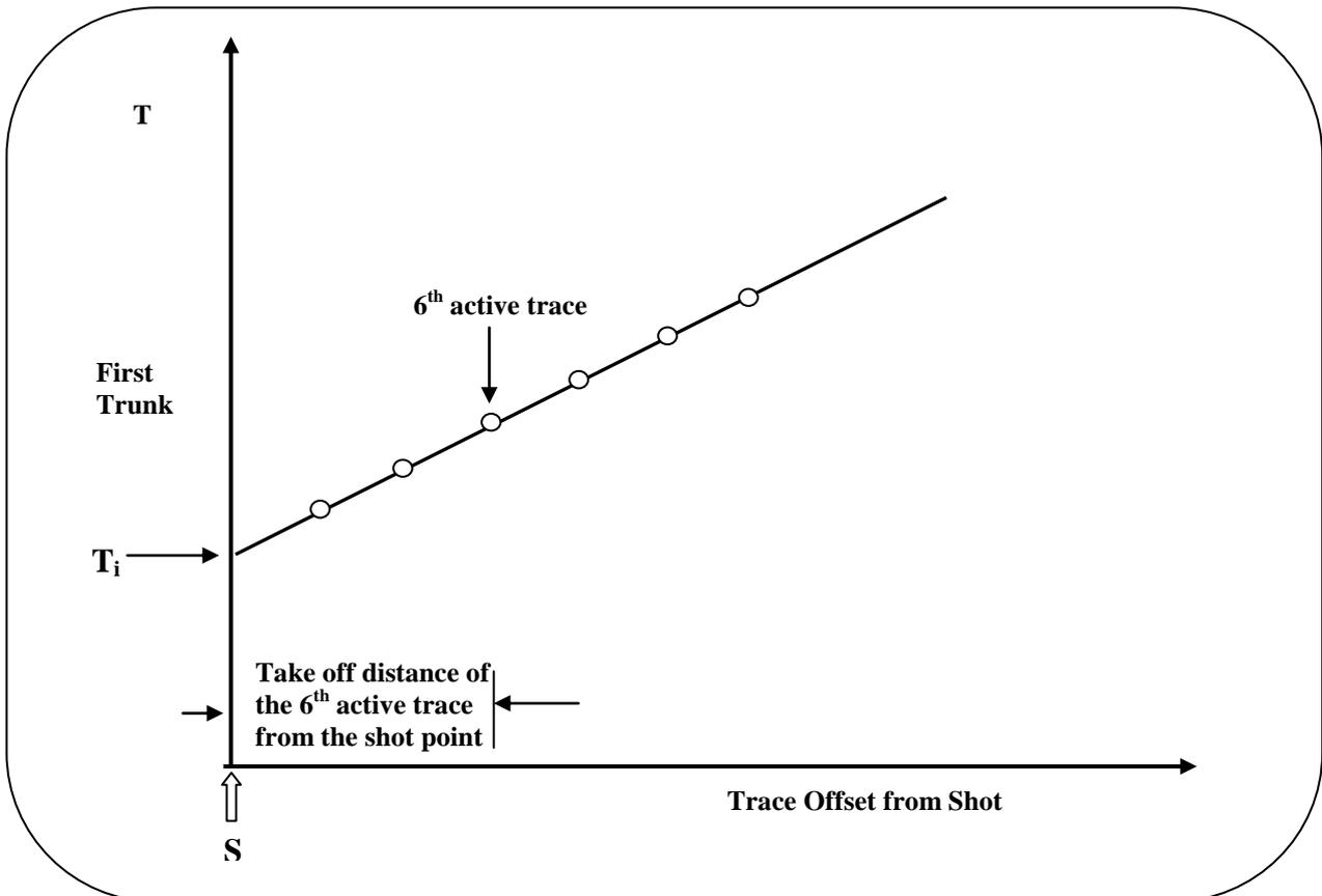
**Fig. 3: Time break versus trace offset plot for a single shot**
