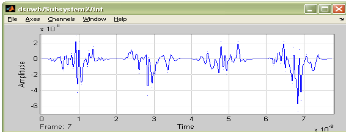
Figure 16: Vector scope display of the output of the 'Integrator'
