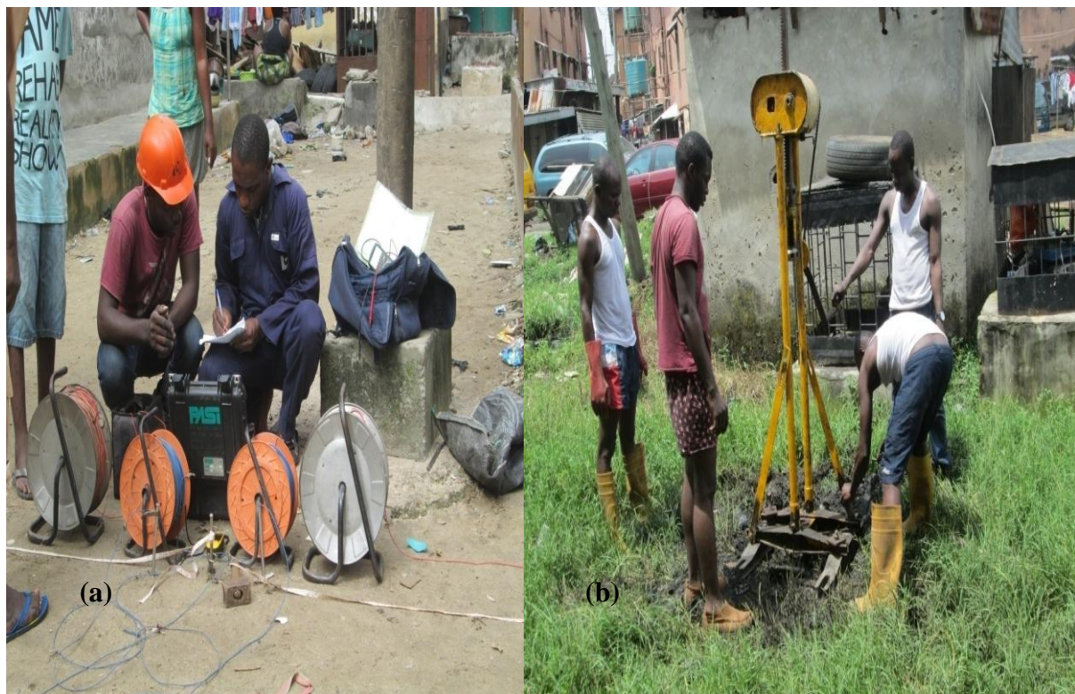
Plate 2: (a) Field Staff, PASI 16GL resistivity meter and its accessories (b) Dutch Cone Penetrometer
