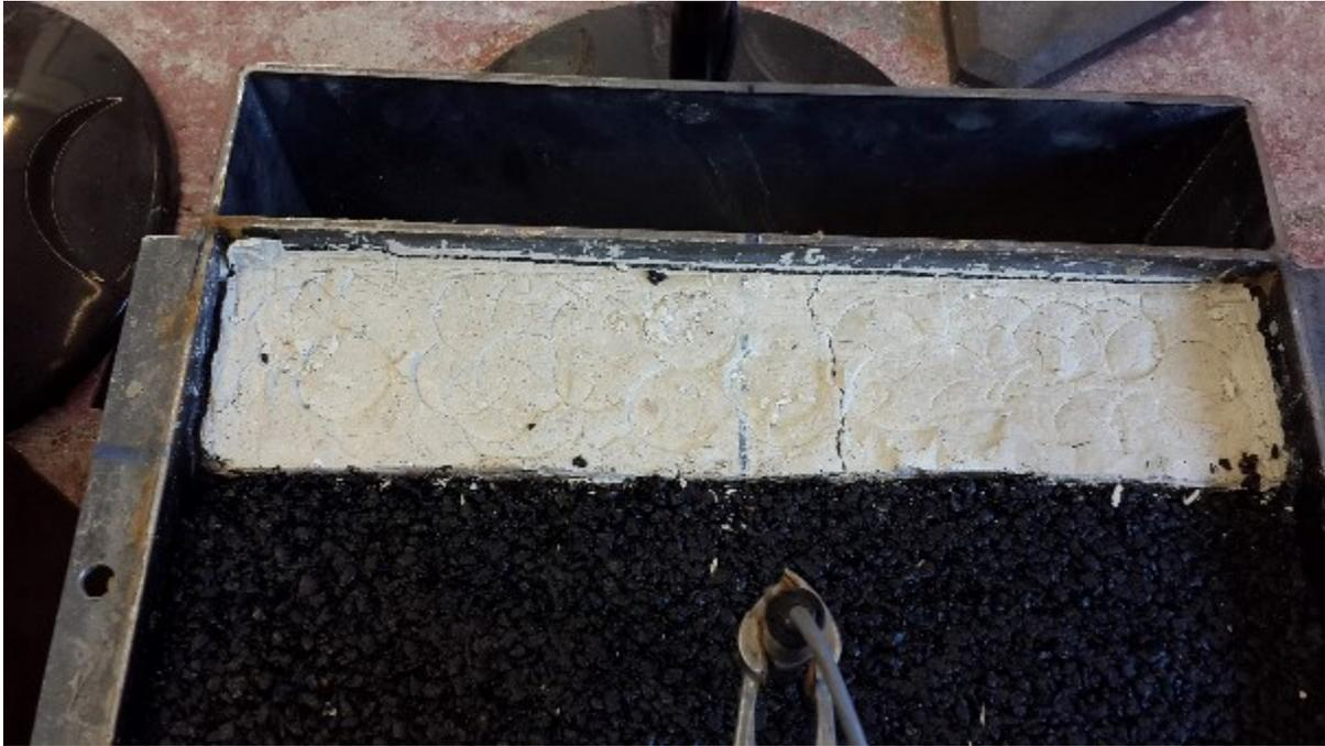
**Figure 8** Illustration of a cross sectional crack on shoulder of a test section
