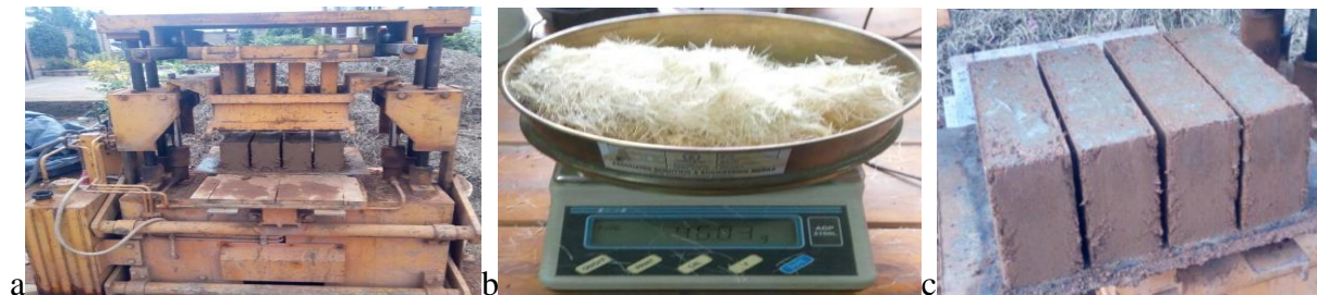
Figure 4: Hydroform machine (a), sisal fibers (b), and Mud reinforced bricks samples (c)
