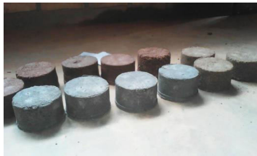
Figure 2: Pavers from plastic wastes and sand
