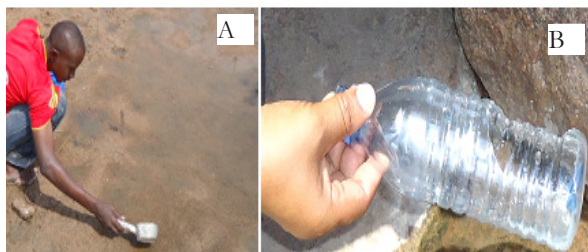
Figure 2. The use of an improvised dipper - a standard dipper and B-Improvised empty 350 ml sized plastic bottle of water dipper
