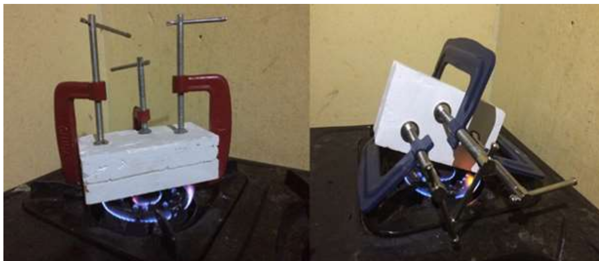
Figure 2: packed silicone in the mold and heating of the mold with gas flame
