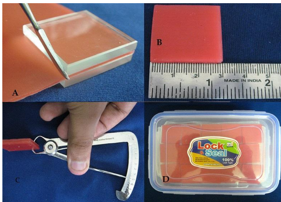
Figure 3: Sample preparation: (A) cutting of wax sample using carver; (B) wax sample measuring 30x30mm; (C) measuring thickness of wax sample using wax gauge; (D) samples stored in air-tight container
