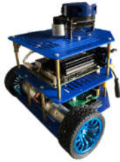
Figure 3. Bveeta Mini Type R-007 mobile robot with ROS framework.
