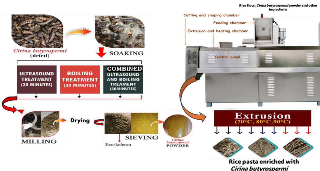
Figure 2. Flow diagram of rice pasta enriched with Cirina butyrospermi powder under different treatment methods and extrusion temperature
