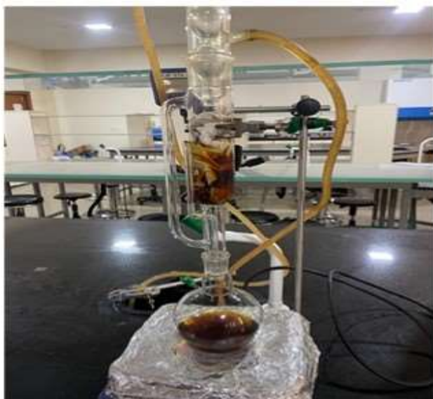
Figure 3: Extraction of crude oil from SACHPC Filter
