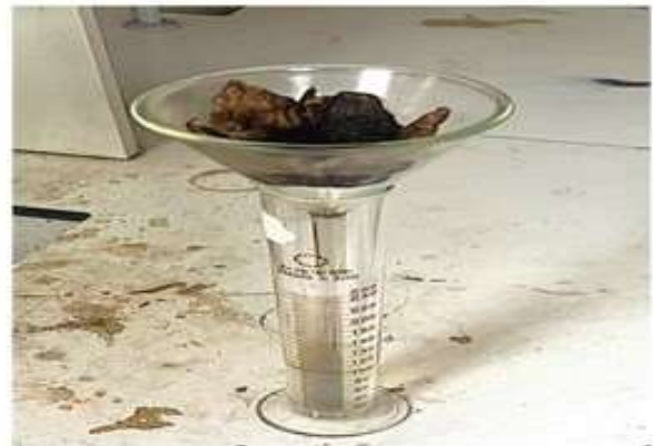
Figure 2: Filtration of crude oil solution using SACHPC filter.
