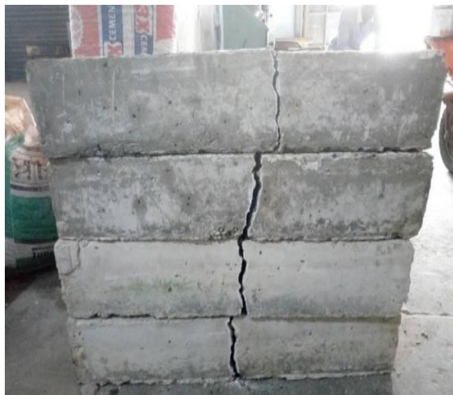
Figure 7: Failure mode of the unreinforced concrete beams containing metakaolin
