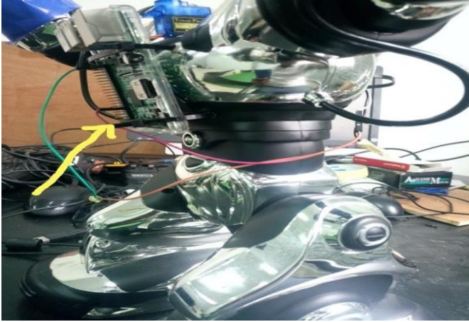
Figure 4: The hacking process involved bypassing the in-built Robosapiens microcontroller (shown in the image) and installing our own raspberry pi controller.
