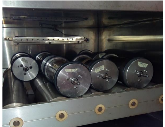
Figure 6: Cells in the roller oven for thermal analysis.
