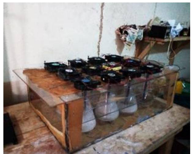
Figure 4: Arrangement of apparatus for the Modified Chappelle test.
