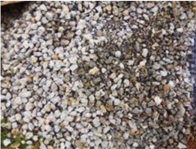
Figure 1: Crushed concrete reduced into coarse aggregate sizes.
