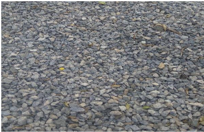
Figure 1: Conventional coarse aggregate (granite).
