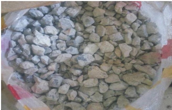
Figure 2: Recycled coarse aggregate (laboratory tested specimens).
