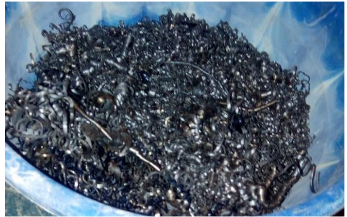
Figure 4: Lathe waste steel fibre.
