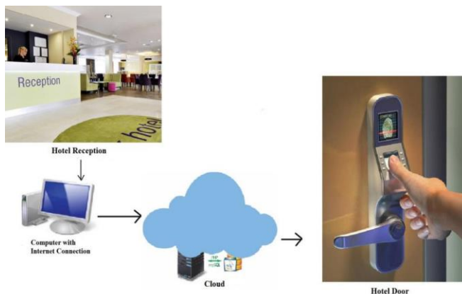
Figure 1: Schematic diagram of the IoT controlled smart door system.
