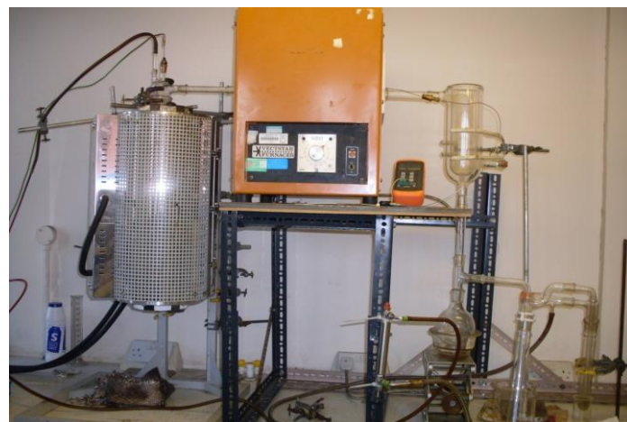
1 = primary reactor, 2 = secondary reactor, 3 = dry ice condenser, 4 = oil pot 5 = secondary condenser, 6 = scrubber
