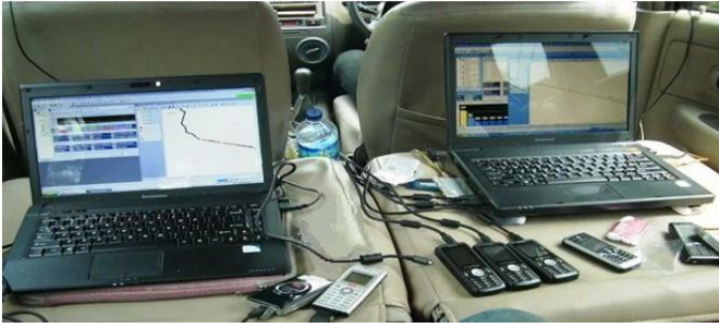
Fig. 1: Experimental setup showing measurement equipment inside a drive test vehicle.
