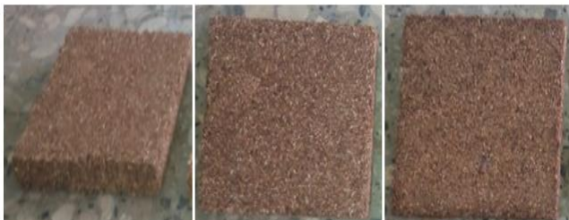
Plate 1: Photographs of PBR Bounded Particleboards fabricated: C1, C2 and C3.
