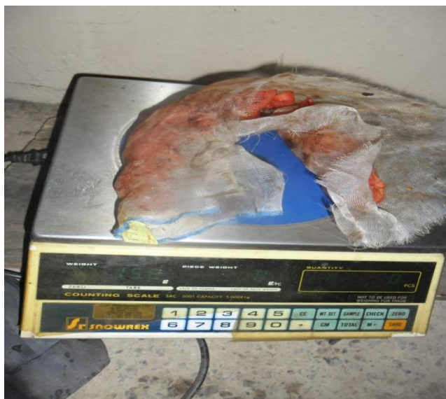
Plate IV: Monitoring the moisture loss of labelled tomato samples at every 1 hour interval of drying.
