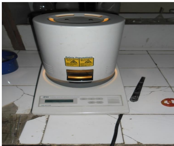
Plate III: Moisture meter at work used in determining the initial and final moisture content of the samples.
