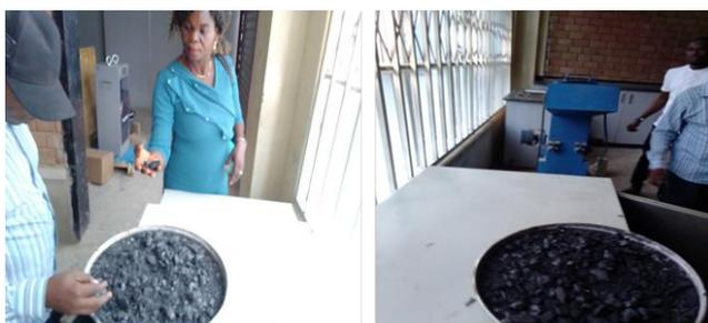
**Figure 1:** Laboratory-produced sodium silicate from rice husk ash after oven drying
