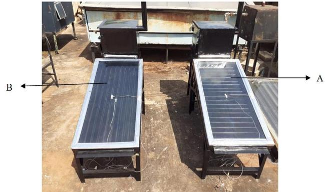
**Figure 1A:** Experimental layout of the Two V-groove SAHs
