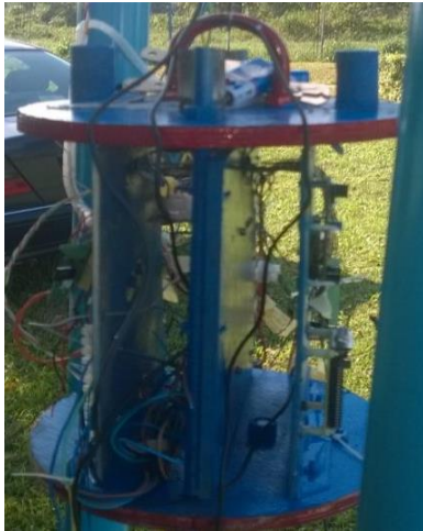
Figure 10: The IMU Based autopilot flight module with GPS tracking station
