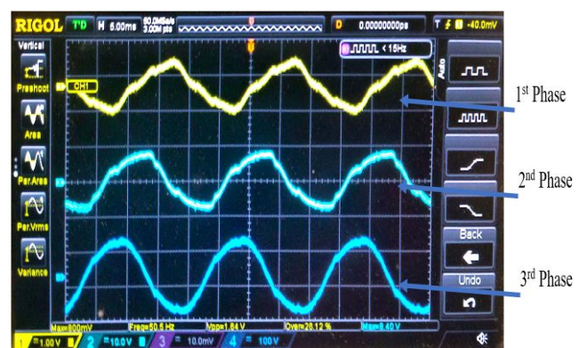
Figure 6: Steady-state phase-voltage under purely inductive load (3-φ, 3-h.p induction motor)
