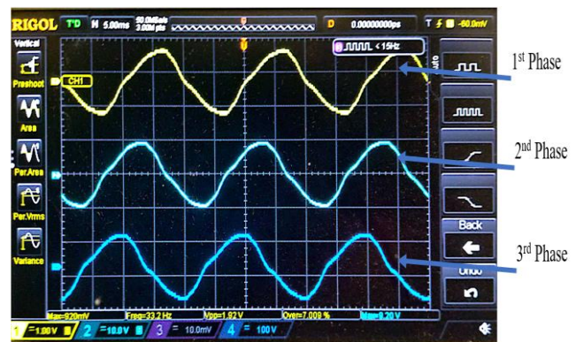
Figure 5: Steady-state phase-voltage under purely resistive loads (three - 200W bulbs)
