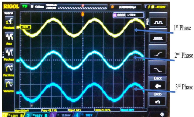
Figure 13: Steady state line current under resistive loads (three - 200W bulbs)
