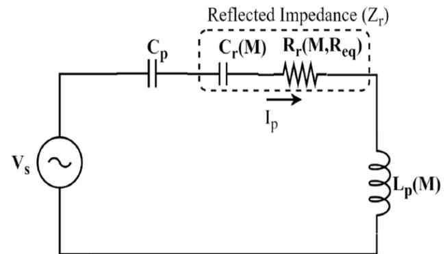
**Figure 4:** Simplified equivalent circuit of SLC architecture [30]
