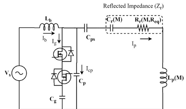
**Figure 5:** Simplified circuit of high-gain LCL architecture [20]
