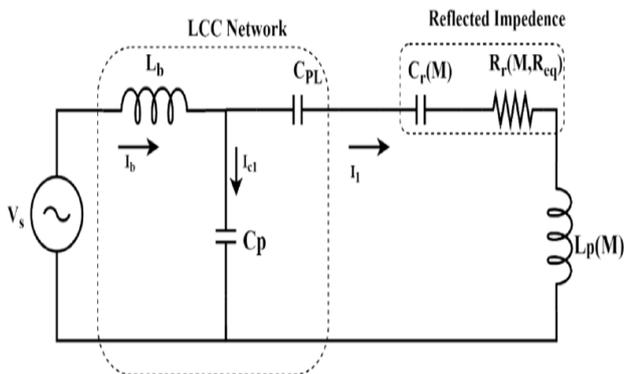
**Figure 3:** An equivalent circuit illustration of LCL architecture [30]
