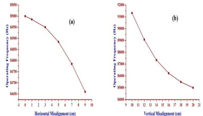
**Figure 6:** Operating frequency versus coil misalignment [67] (a) Horizontal misalignment of coils, (b) Vertical misalignment of coils
