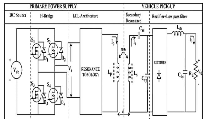
**Figure 2:** H-bridge inverter based wireless charger system [30, 61]
