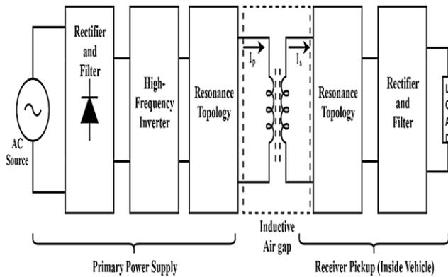
**Figure 1:** Schematic of an inductive EV charger system [30].
