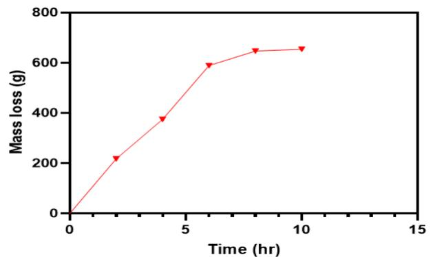
**Figure 1:** Mass loss values of Aluminum in 1.0 M NaOH without *Gk* against time (hr)
