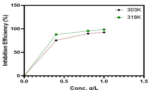
**Figure 3:** Inhibition Efficiency of aluminum alloy in 1.0M NaOH at different temperatures
