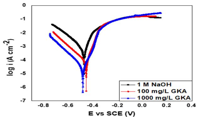
**Figure 8:** Potentiodynamic polarization (PDP) plots of Aluminum in the presence of *Gk* in 1 M NaOH environment
