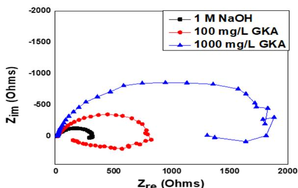
**Figure 9:** Electrochemical impedance spectra plots of Aluminum with *Gk* in 1 M NaOH environment
