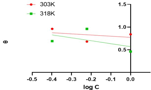
**Figure 7:** Temkin isotherm for adsorption of *Gk* on aluminum alloy in 1.0M NaOH
