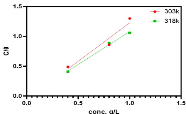
**Figure 4:** Langmuir isotherm for adsorption of Gk on aluminum alloy in 1.0M NaOH
