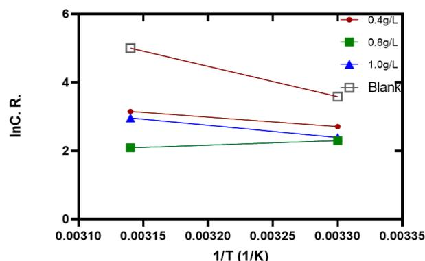
**Figure 5:** Plot of  $\ln C.R.$  against  $1/T$  for Aluminum alloy corrosion in 1.0M NaOH (Blank) and inhibited solutions at various concentrations of Gk
