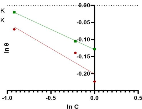
**Figure 6:** Freundlich isotherm for adsorption of *Gk* on aluminum alloy in 1.0M NaOH
