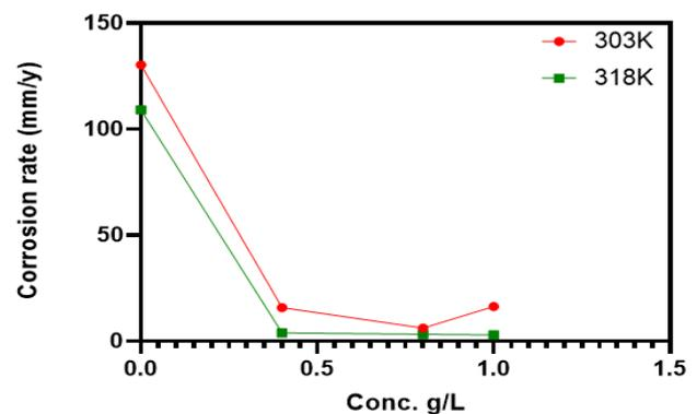
**Figure 2:** Corrosion rate variation of aluminum alloy in 1.0M NaOH at different temperatures
