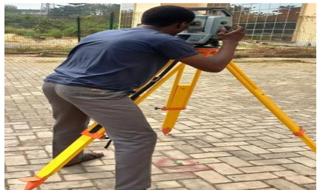
**Figure 5:** Total station setup on a monitoring point
