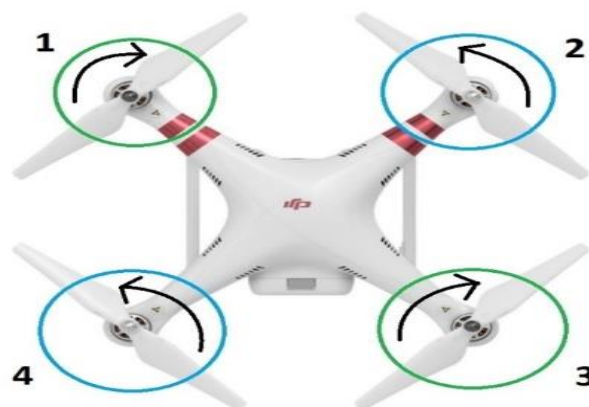
Figure 1: Motors directions of the quadcopter [Source: https://www.dronezon.com/learn-about-drones-quadcopters/how-a-quadcopter-works-with-propellers-and-motors-direction-design-explained/ ]
