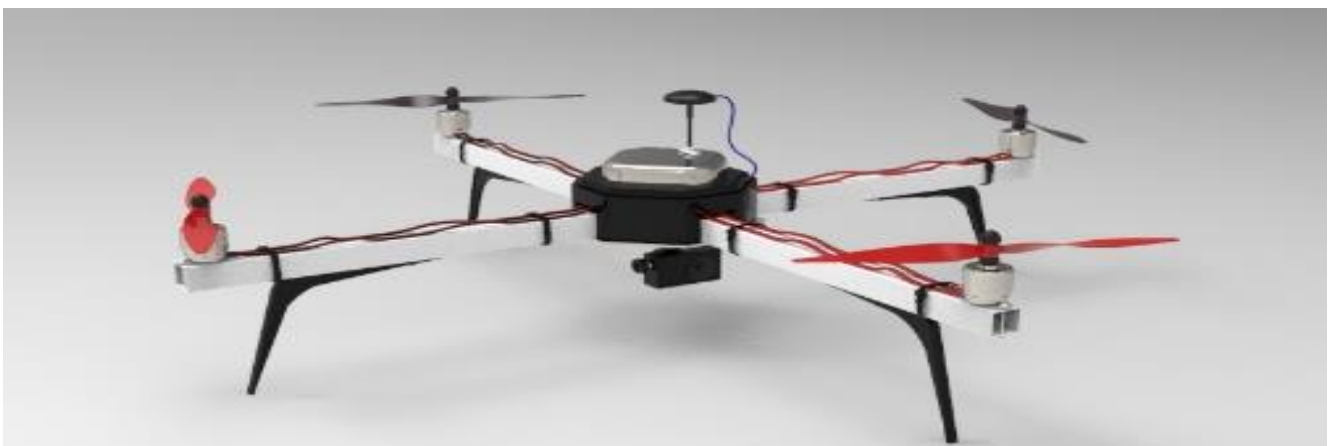
Figure 3: Initial CAD design of the drone made in Autodesk maya software before actual construction of the UAV
