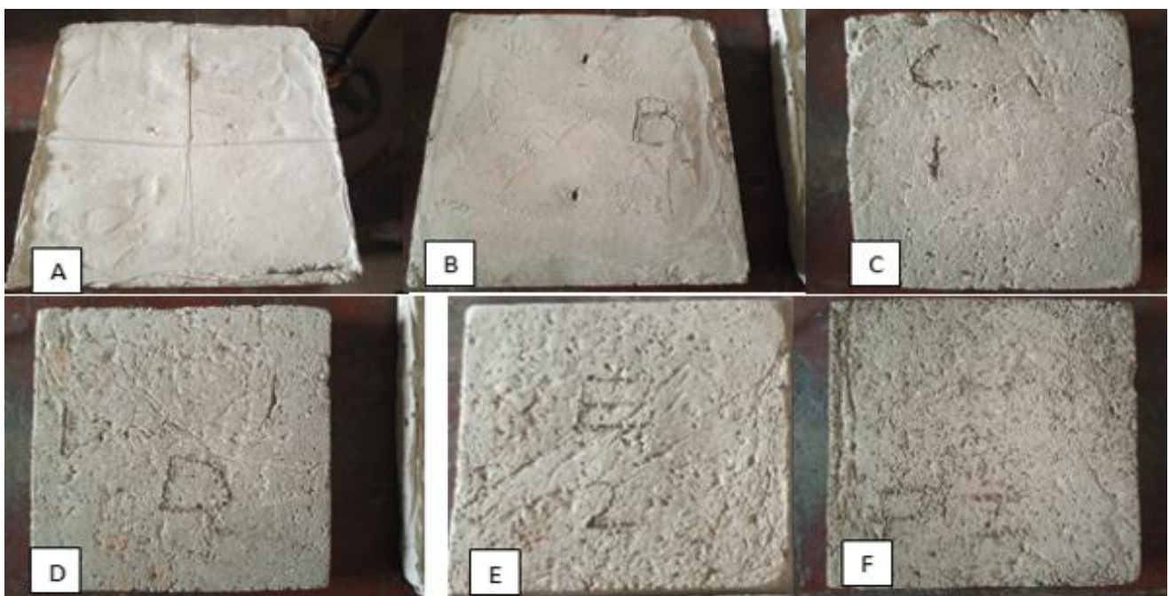
Figure 8: PKS/Cement ratio A (0:100), B (20:80), C (40:60), D (50:50), E (60:40) and F (80:20)
