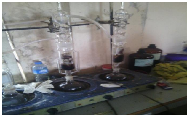
Figure 1: Experimental setup for the extraction of oil from tar sand
