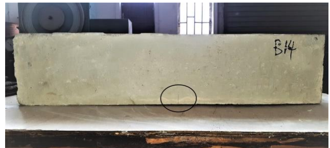
Figure 4: Picture showing first crack on the hollow cored beams that emanated due to the point load on a Type 3 Beam.
