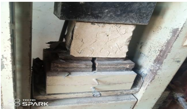
Figure 3: Loading the equipment for compressive strength measurement
