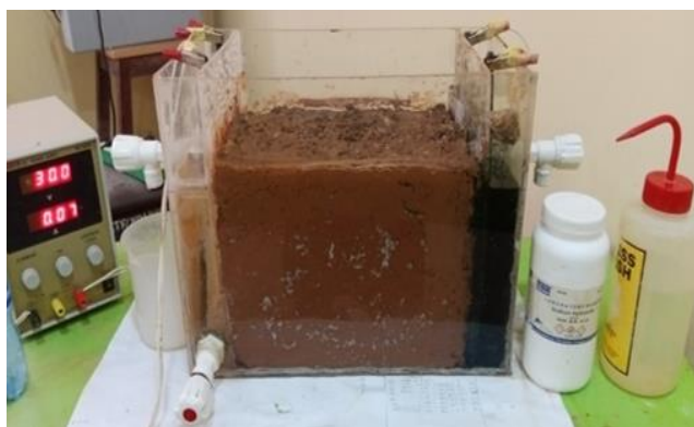
Figure 2: Filter Media Enhanced EKR Setup for Crude-oil Contaminated Soil
