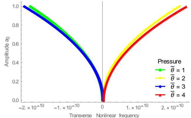
**Figure 2a:** Transverse amplitude-frequency response at void fraction=0.3 , mixture quality = 0.00037088;  $Teb=0.1$ ;  $Pr = 0.05$ ;  $\theta b=1,2,3,4$ ;
