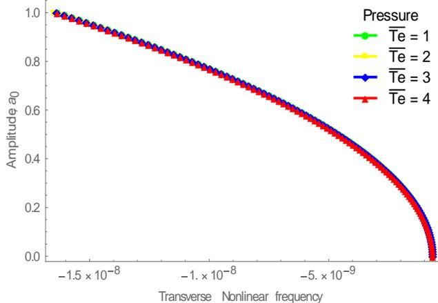
**Figure 3a:** Transverse amplitude-frequency response at void fraction=0.3, mixture quality = 0.00037088;  $\theta_b=1.2$ ;  $Pr_b=0.05$ ;  $T_{eb}=1,2,3,4$ ;
