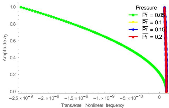
**Figure 1a:** Transverse amplitude-frequency response at void fraction=0.3 , mixture quality = 0.00037088;  $\theta b=1.2$ ;  $Teb=0.1$ ;  $Pr = 0.05; 0.10; 0.15; 0.20$ ;
