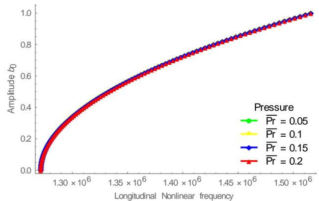
**Figure 1b:** Longitudinal amplitude-frequency response at void fraction=0.3 , mixture quality = 0.00037088;  $\theta b=1.2$ ;  $Teb=0.1$ ;  $Pr = 0.05; 0.10; 0.15; 0.20$ ;
