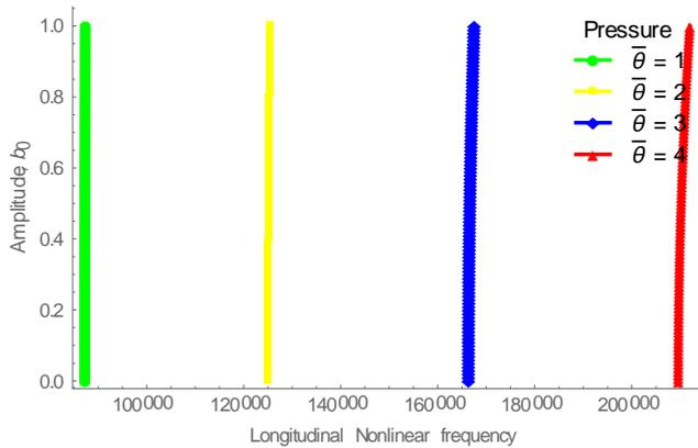
**Figure 2b:** Longitudinal amplitude-frequency response at void fraction=0.3 , mixture quality = 0.00037088;  $T_{eb}=0.1$ ;  $Pr = 0.05$ ;  $\theta_b=1,2,3,4$ ;
