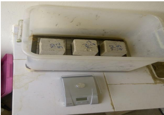
Figure 2: Experimental set up for capillary absorption measurement
