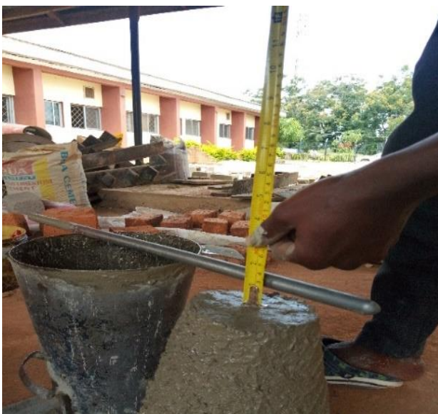
Figure 3: Measurement of the Slump Value
