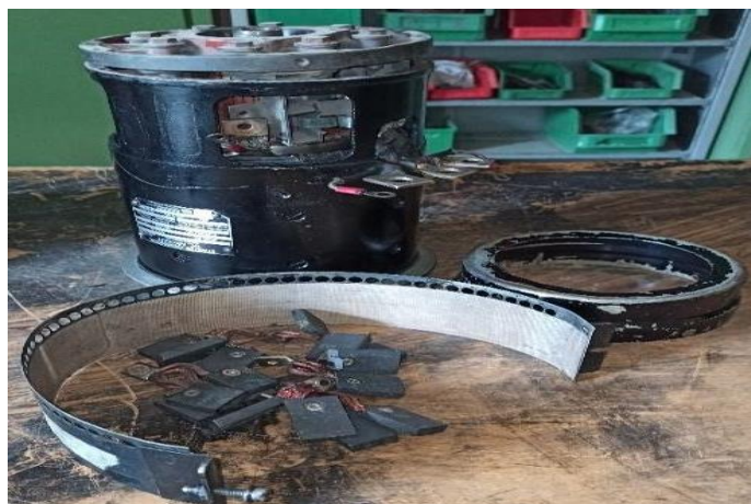
Figure 5: Starter Generator Top-level Overhaul [10].
