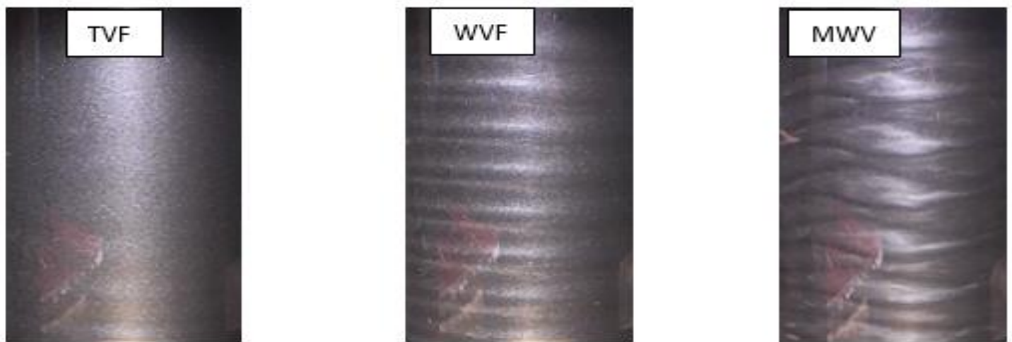
Figure 13: Onset of different flow regimes in the absence of magnetic field at 0.002% nanoparticle volume fraction.
