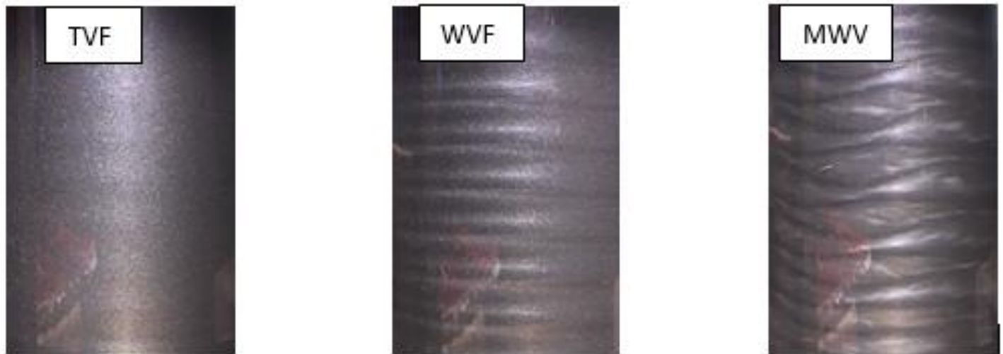
Figure 12: Onset of different flow regimes in the presence of magnetic field at 0.002% nanoparticle volume fraction.
